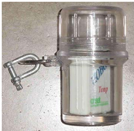
Figure 2.3a Water temperature logger inside polycarbon case
