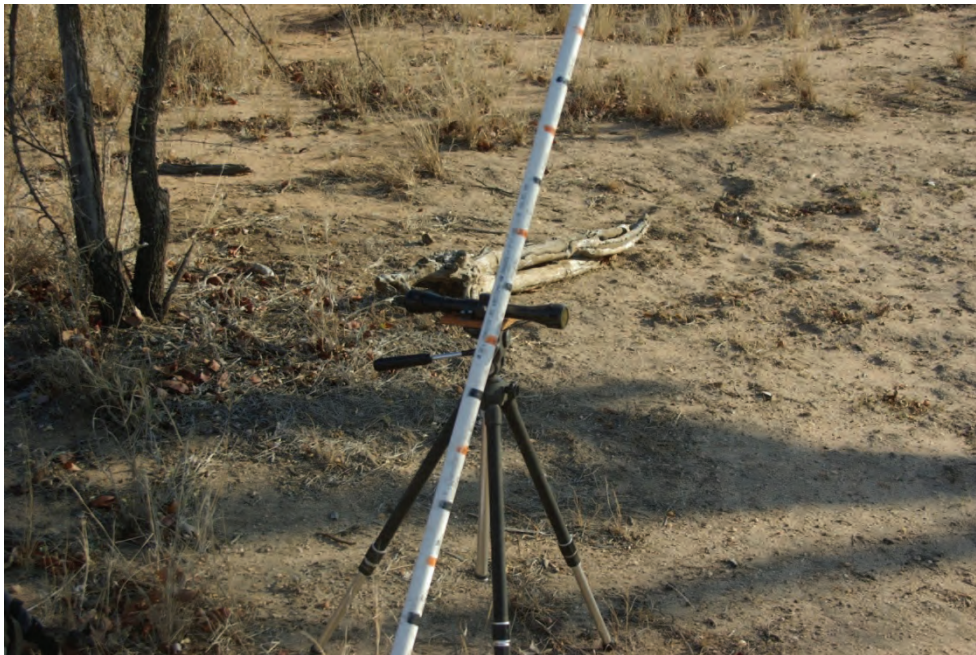
Figure 3.3: The theodolite and measurement staff used during measurements of pan depths in the Kruger National Park.
